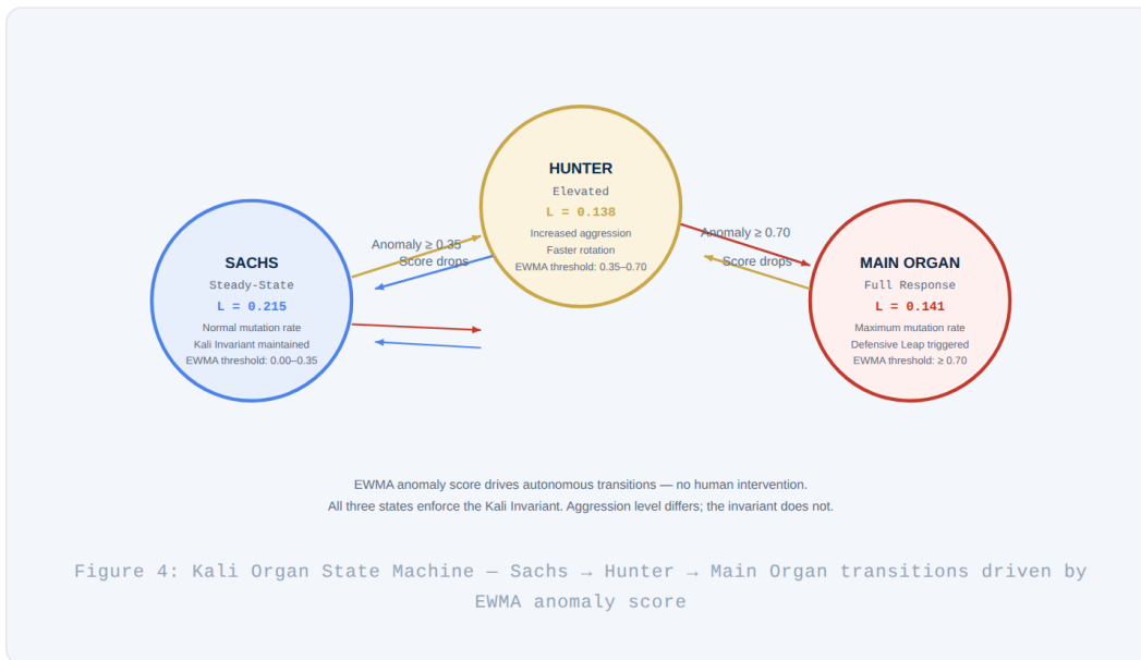
Figure 4: Kali Organ State Machine — Autonomous transitions driven by EWMA anomaly score
